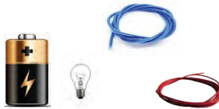
Figure 7.3. Things needed to make a circuit.
