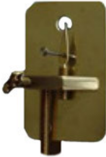
Figure 1.2 Leeuwenhoek's simple microscope
