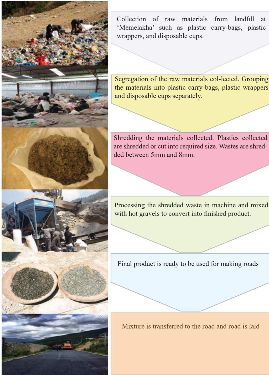
Figure 2.2 illustrates the operations process followed in the Green Road, Bhutan.
