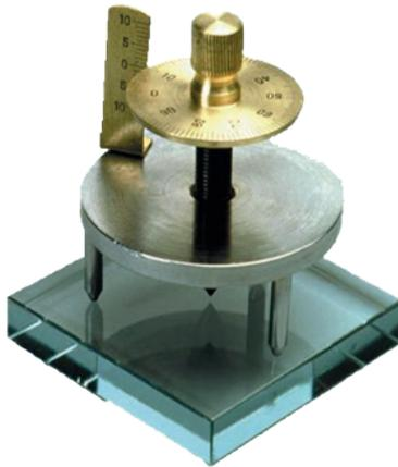
Figure 8.1. Measurement of plane surface of glass slab.
