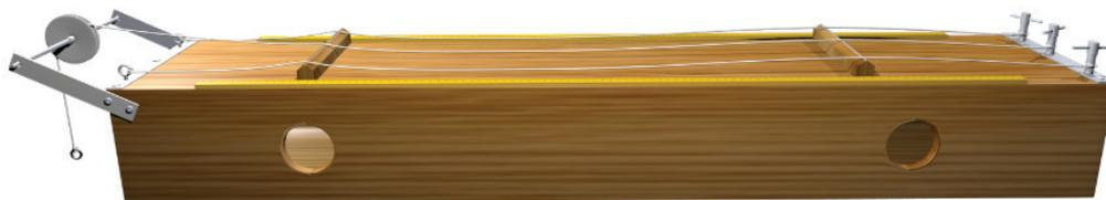
Figure 6.21. Sonometer.
