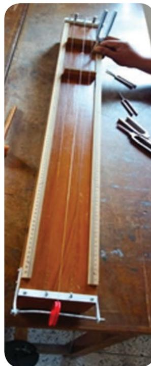
Figure 2.1. Experimental set up for sonometer.
