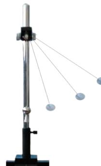
Figure 6.26. Simple pendulum.
