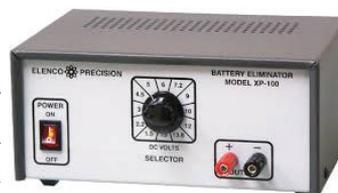
Figure 6.11. Battery eliminator.
