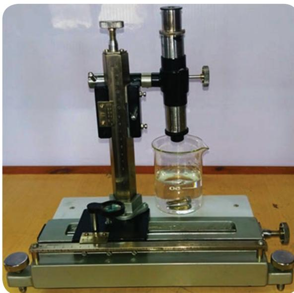
Figure 10.1. Experimental set up for travelling microscope.
