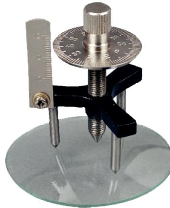
Figure 8.2. Measurement of a curved surface.
