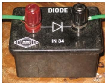
Figure 6.27. Semiconductor diode.
