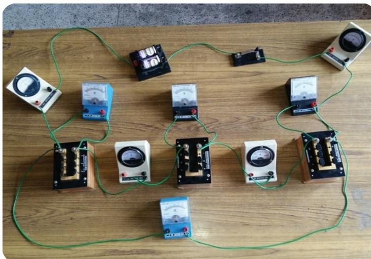
Figure 5.3. Combination of resistors in series.
