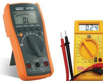
Figure 6.8. Multimeter.
