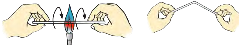
Figure 6.5. Bending glass-tube in non-luminous flame.
