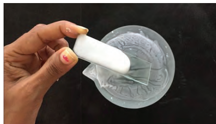
Figure 6.20. Preparation of TLC Plate.
