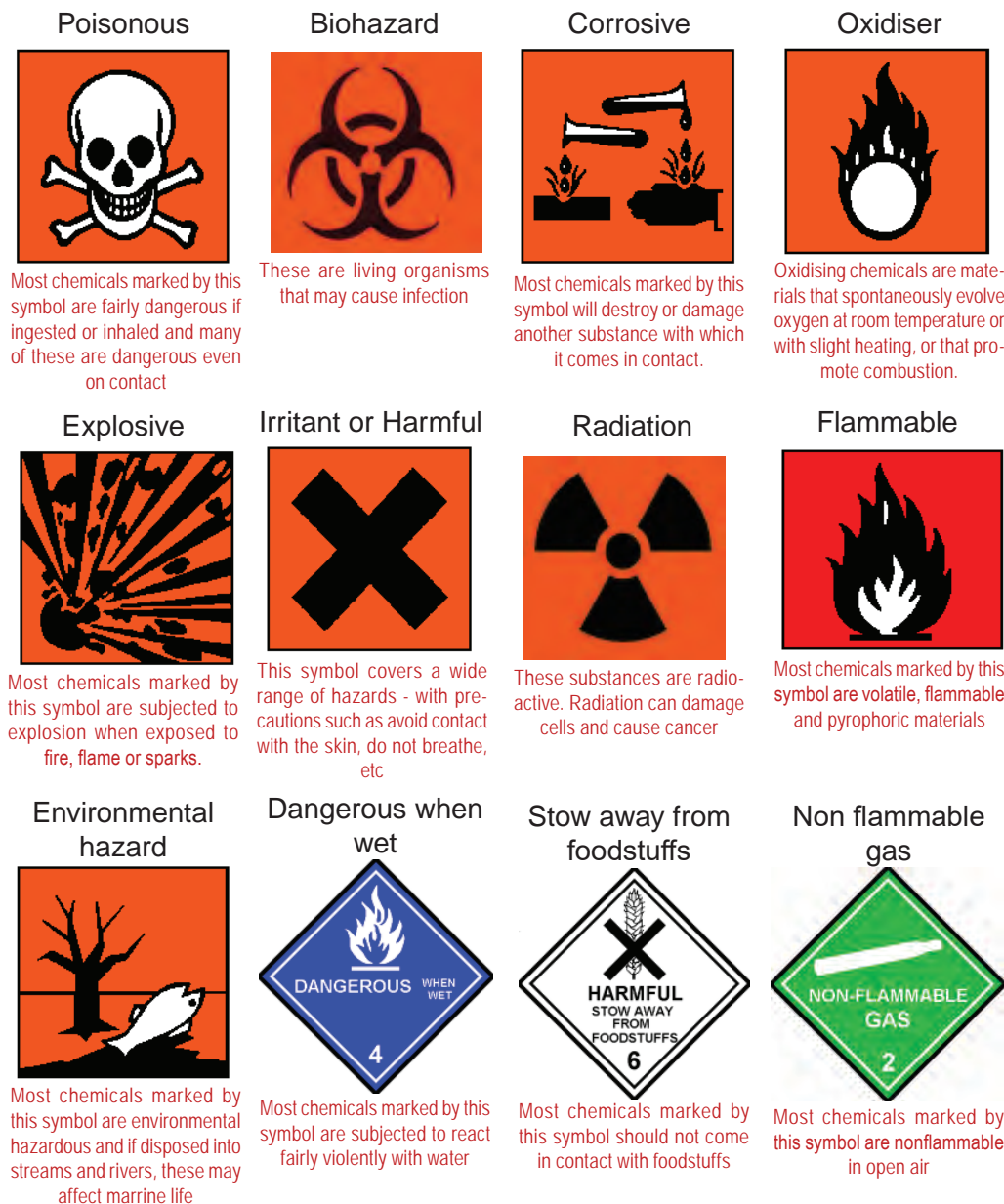
Figure 4.1. Safety warning signs.
