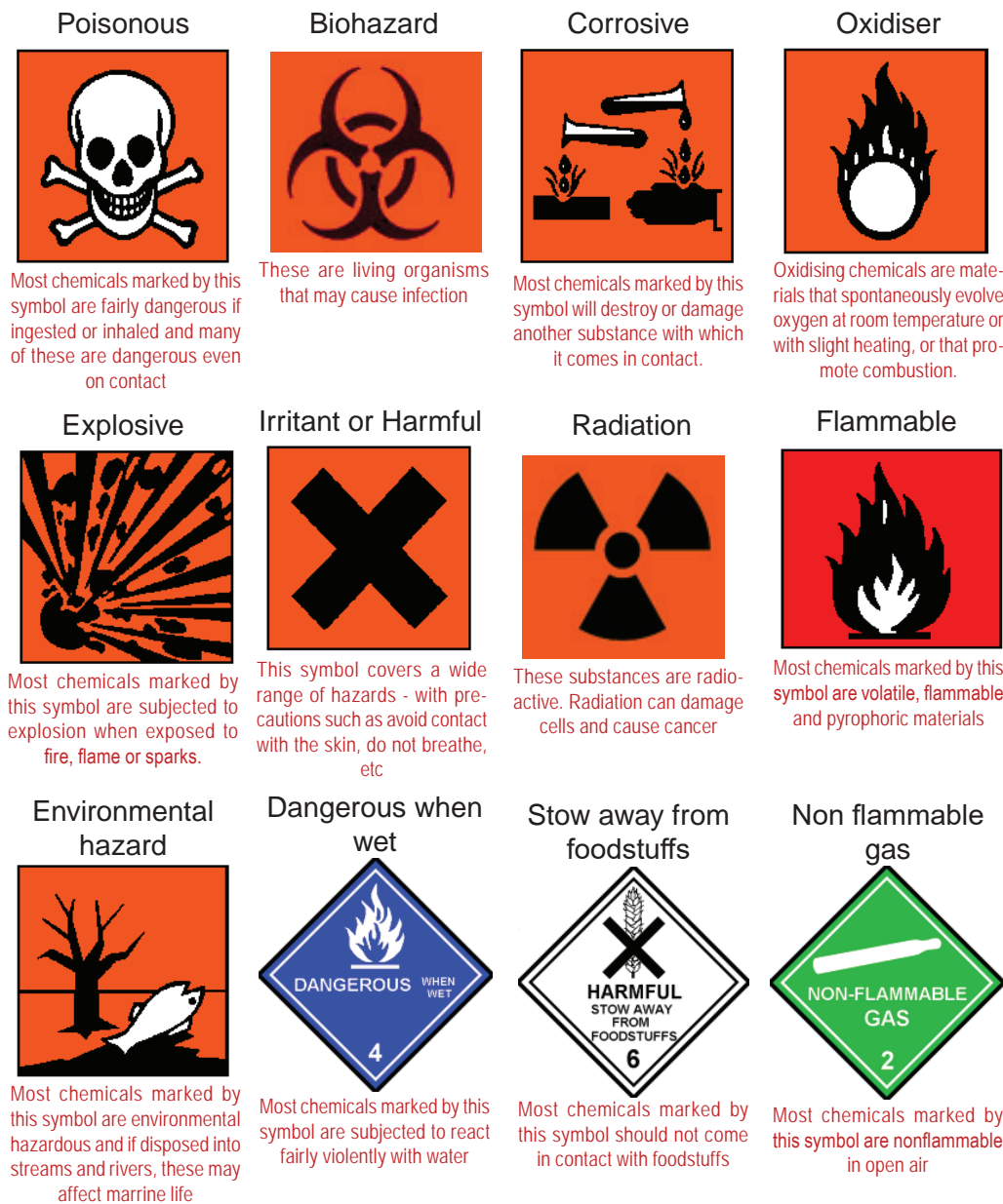
Figure 4.1. Safety warning signs.
