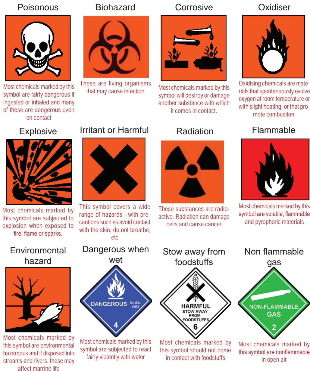
Figure 4.1. Safety warning signs.
