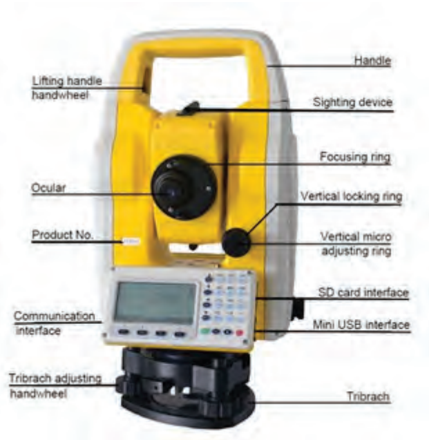
Fig. 2.11 Labelled Total Station
