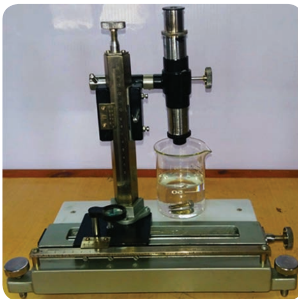
Figure 10.1. Experimental set up for travelling microscope.
