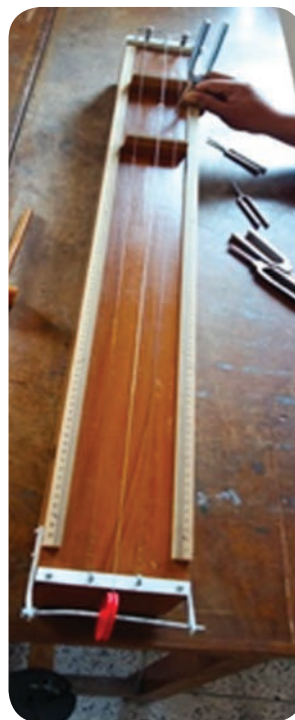
Figure 2.1. Experimental set up for sonometer.
