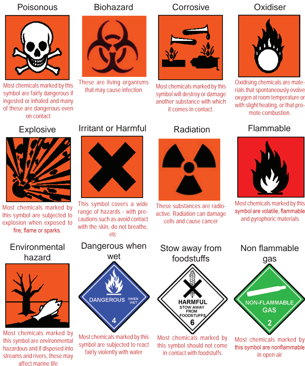
Figure 4.1. Safety warning signs.
