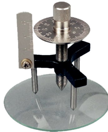
Figure 8.2. Measurement of a curved surface.
