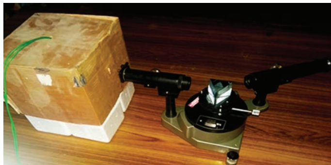
Figure 6.2 Diagram showing spectrometer with prism and source of light
