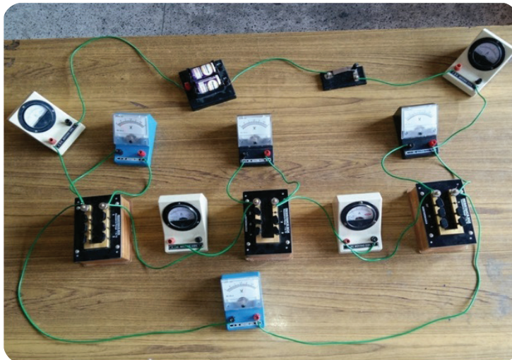
Figure 5.3. Combination of resistors in series.
