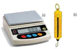
Figure 5.4. (a) Digital balance (b) Spring balance.
