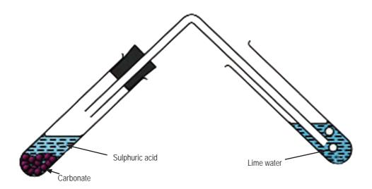
Figure. 8.1. Lime water test.
