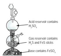
Figure 6.15. Internal structure of Kipp's apparatus.
