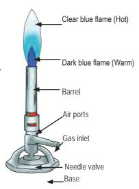
Figure 6.12. Parts of bunsen burner.
