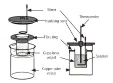
Figure 1.1. Calorimeter.
