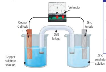
Figure 3.1. Electrochemical cell.
