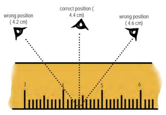
Figure 5.6. Position of eye while measuring.
