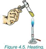
and mouth of the test tube pointed away from people. Always use a minimum quantity of substance for heating.
