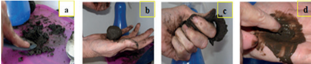
Figure 10.10. Procedure for determining soil texture
